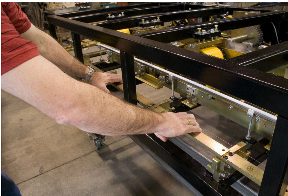
Figure 63: Right Side Fixed Mount Rail Adjustment
