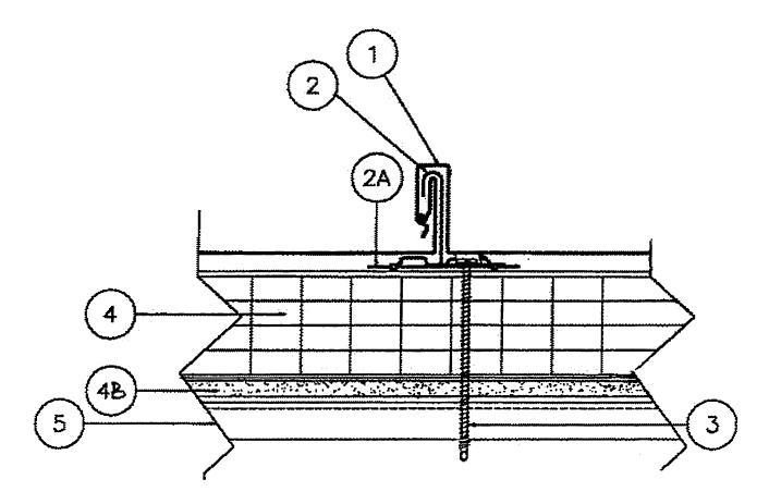
1. Metal Roof Deck Panels\* — No. 24 MSG min thickness coated steel. Panel width 18 in. max., 10 in. min. ribs height 1-3/4 in. at female side. Panels continuous over three or more clips with no end laps. A bead of sealant may be used at panel side joints.
