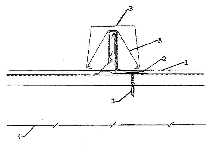
1. Metal Roof Deck Panels\* — 0.032 in. thick aluminum or No. 24 MSG min thickness coated steel. Panels 10-1/2 in. wide, 1-3/4 in. high at the ribs. Panels continuous over two or more spans. A bead of sealant may be used at panel side joints.
