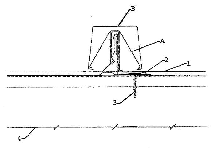
1. **Metal Roof Deck Panels** \* — No. 22 MSG or No. 24 MSG min thickness coated steel panels. Panels 12 in. wide, 1-3/4 in. high at the ribs. Panels continuous over two or more spans. A bead of sealant may be used at panel side joints.
