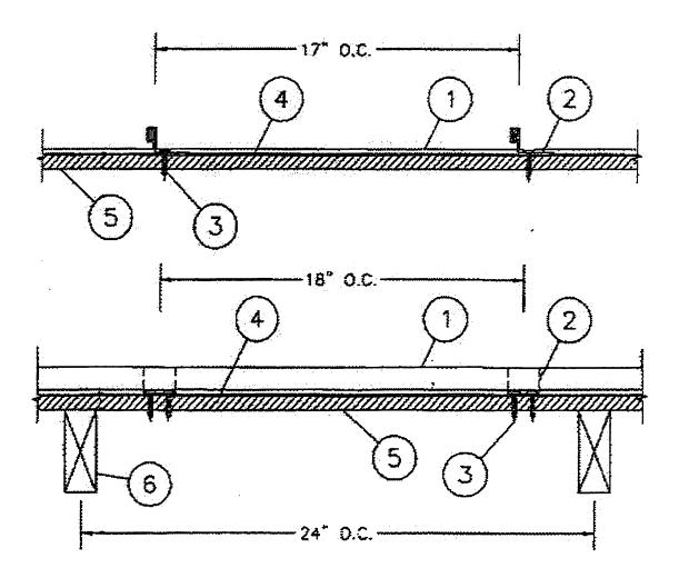
1. Metal Roof Deck Panels\* — 0.0216 in. thick copper (16 oz). Max panel width 17 in., rib height 1 in. Panels continuous over two or more spans with no end-lap.
