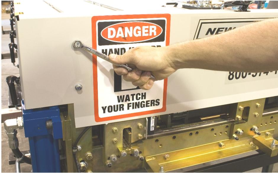
*Figure 66: Removing Shear Cover*
