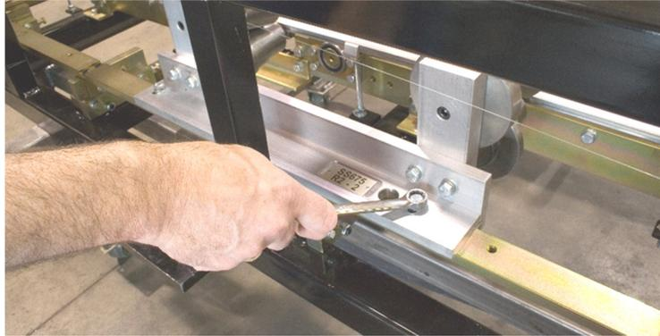
**Figure 53: Removing Tooling Rails**
